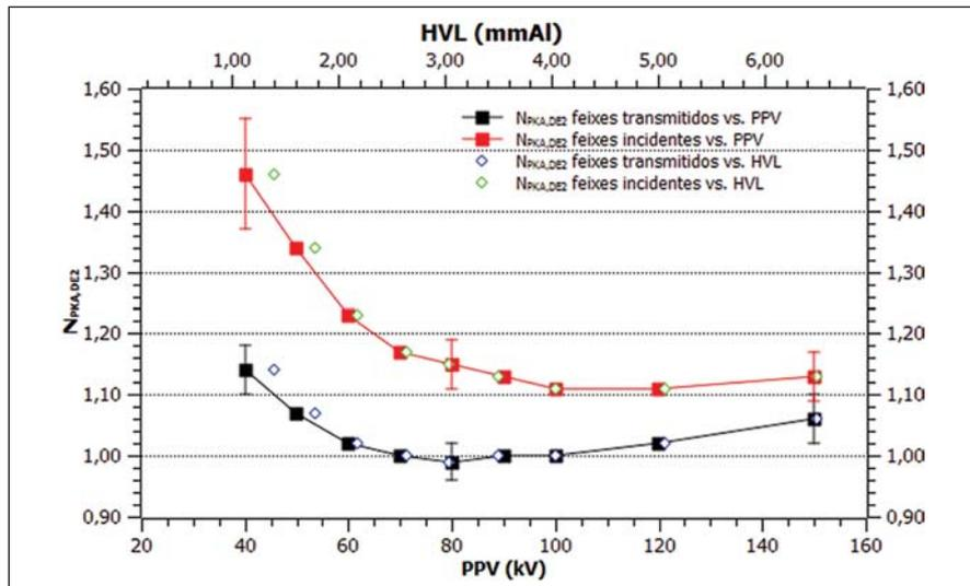
Figure 3. Energy dependence of the DE2 meter calibration for incident and transmitted beams of the RQR series (Table 4), measured against the standard 30 cm<sup>3</sup> chamber, as a function of PPV and of the 1st HVL.
