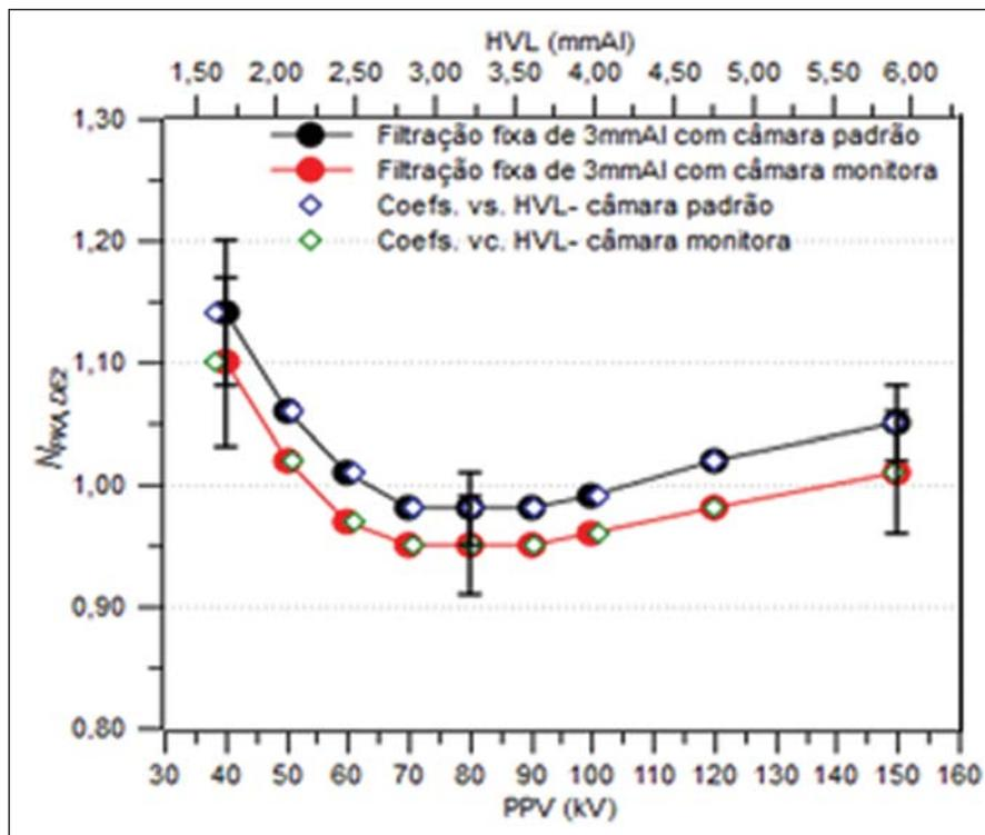
Figure 4. DE2 meter calibration coefficients for beams with 3 mmAl fixed filtration, utilizing as reference the PTW 30 cm<sup>3</sup> chamber (black circles) or the PTW monitor chamber (red circles), both as a function of the PPV and HVL.
