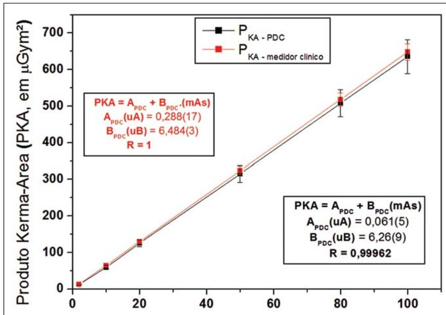
Figure 6. Variation of  $P_{KA}$  values as a function of the current-time product (mAs), for the PDC and the clinical IBA meter (linearity curve).
