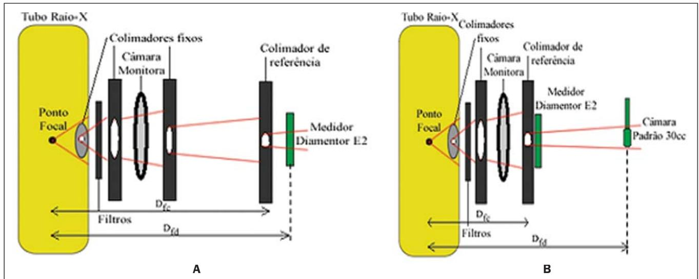
**Figure 1.** Geometry utilized to calibrate the PTW DE2 meter (A) by the substitution method against the standard 30 cm<sup>3</sup> chamber, for incident beams, and (B) by a tandem type method for beams transmitted by the meter. The additional filtration for the RQR series was previously determined. D<sub>fc</sub> is the focus-collimator distance (93.5 cm on A and 33.5 cm on B) and D<sub>fd</sub> is the focus-detector distance (99.5 cm).
