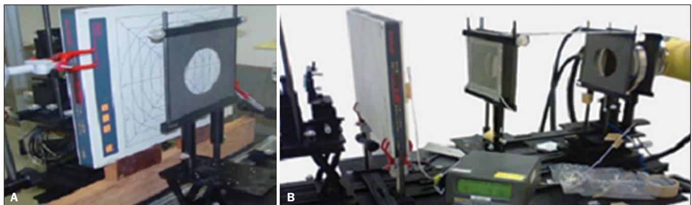
**Figure 2. A:** Experimental assembly in laboratory for PDC meter calibration for incident beams, utilizing the 30 cm<sup>3</sup> chamber as reference. **B:** Assembly for calibration of the DE2 meter against the previously calibrated PDC meter, for beams transmitted through the DE2 meter.
