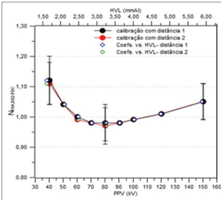
**Figure 5.** Results of the DE2 meter calibration against the calibrated PDC meter, for beams with 3 mmAl fixed filtration, at two different distances (65.5 cm and 42.3 cm) between focus and P<sub>KA</sub> meter, ( $N_{P_{KA},DE2-PDC}$  vs. PPV, HVL).
